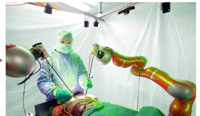
The operating scenario. Environmental cameras are supervising the scene and the robots are cooperating with the surgeon.
