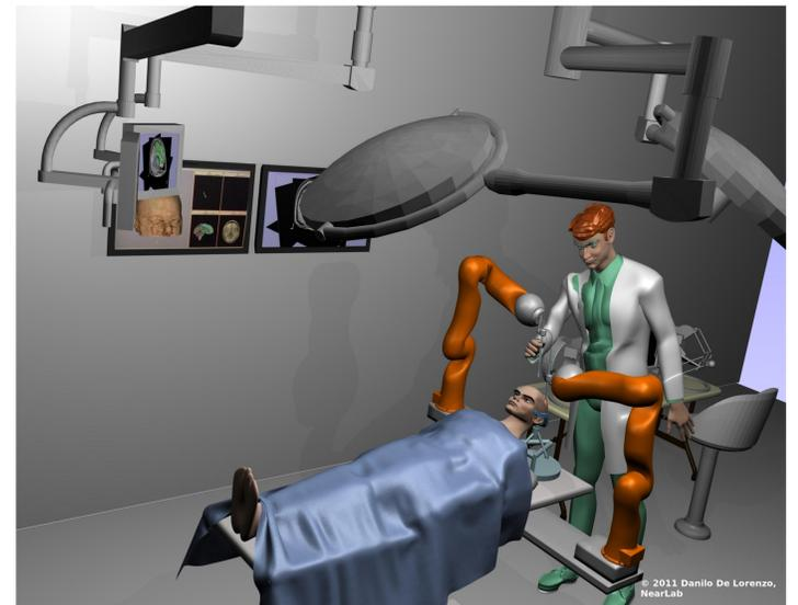
The ACTIVE scenario: two light weight robots are acting on the brain tissue, assisting the surgeon.
